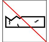
Always inspect the Power-Pad before use, to ensure it is in good condition and free from any cracks, deformations, or damage that may affect its structural integrity.
